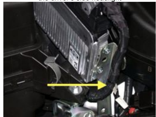
Picture 1C: wire tie to the ECU harness
