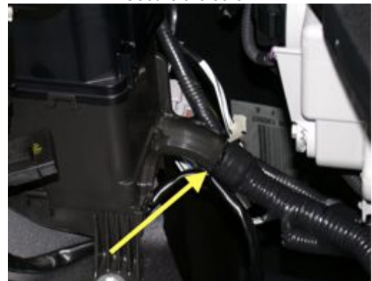
Picture 1B: wire tie to the harness just below the driver's side headlight
