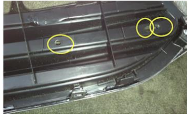
Picture 32A: showing holes from back of grill.
